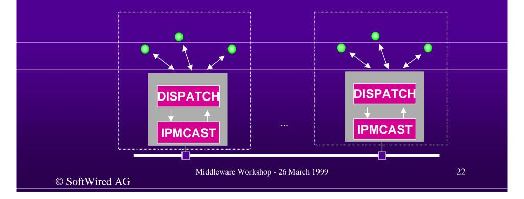
Message Oriented Middlewares **iBus Protocol Stack (3)** DISPATCH DI PATCH RAG Large Data FRAG **FIFO Order FIFO FIFO** ZIP NAK NAK Reliability REACH REACH CRYPT • • • **IPMCAST IPMCAST** Middleware Workshop - 26 March 1999
